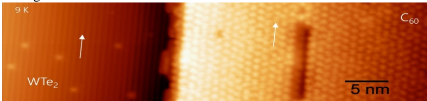
Fig. 2: STM of 1 ML C_{60} on WTe_2 . LUMO, V_s = 1 V, I_T = 10 pA
