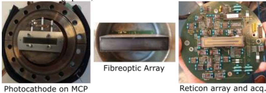
Figure 14 - Legacy SPRED detector design with front end (left), tapered fibreoptic array (middle) and Reticon array with acquisition (right)
